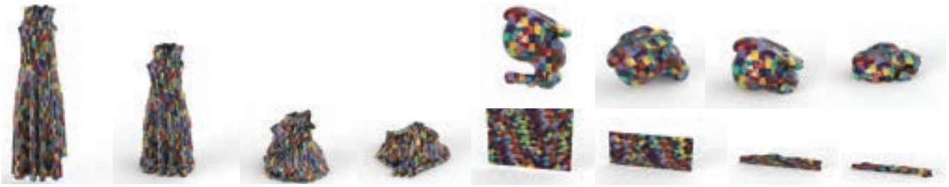
Fig. 9. Patch-based collision culling. Our implementation includes a simple and effective culling modality. The input model is subdivided into patches based on a regular voxelization. Patch BVH facilitates a broad phase culling, which generates a list of overlapping patches. Because intra-patch primitive pairs are pre-built, primitive-level CCD is then followed to compute t_I for all the inter- and intra-patch primitive pairs.
