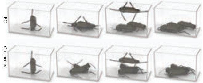
Fig. 11. Rubber helicopters. We simulate three rubber helicopters colliding in a glass tank. This is a fullspace simulation and involves over 150K DOFs and 224K elements. Both IPC and our method produce plausible animations with the guarantee of interpenetration-free. Being a GPU algorithm, our method is over 2,000× faster than IPC.
